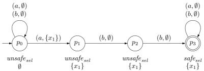
Figure 3: Automaton A for the query selecting a-nodes followed by  $b \cdot b$ . There are two reachable unsafe states of type  $\{x_1\} = \mathcal{V}_1$ ,  $p_1$  and  $p_2$ . The restriction of A to these two states is acyclic, so the selection delay of  $Q_A$  is bounded. It is bounded by 2, since the longest path in this part of the automaton has 2 nodes.
