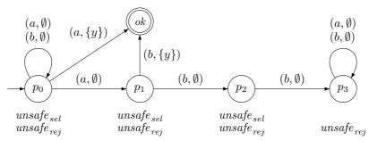
Figure 5: nfa C(A,B) for query dfa A in Figure 3 and trivial universal B. Even though non-deterministic, the ambiguity of C(A,B) is 1, equally to the concurrency of  $Q_{(A,B)}$ .
