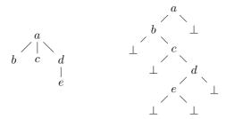
(a) A unranked tree  $t \in \mathcal{T}_{\Sigma}$  (b) The binary tree  $fcns(t) \in \mathcal{T}_{\Sigma_{\perp}}^{bin}$
