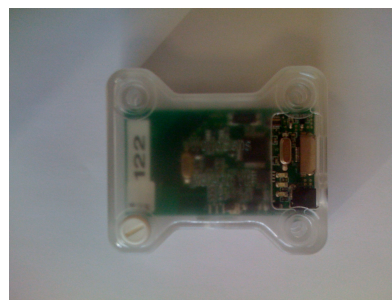
Figure 5: A WSN430 sensor node.
