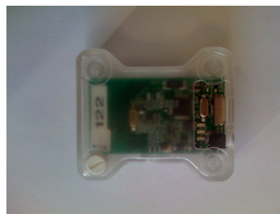
Figure 5: A WSN430 sensor node.
