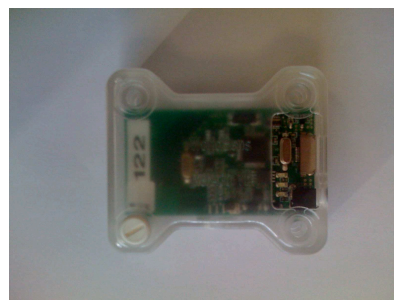
Figure 5: A WSN430 sensor node.
