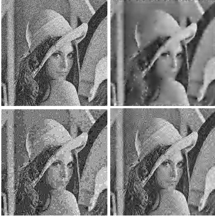
Figure 22: Robustness to noise: qualitative comparison between our new codec, JPEG, and JPEG2000 under the same rate restriction (here 0.27 bpp ). Upper left: Lena (renormalized in the range of values from 0 to 1) with additive Gaussian noise ( mean = 0 , variance = 0.05 ). Upper right: coded/decoded image using the new codec. Lower left: coded/decoded image using JPEG. Lower right: coded/decoded image using JPEG2000.
