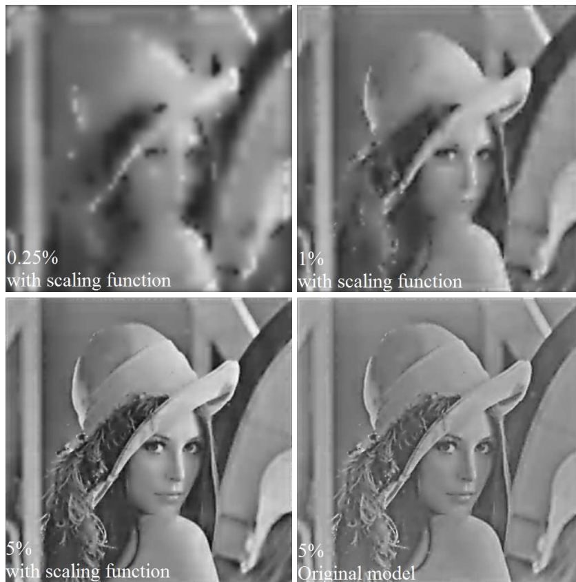
Figure 15: Progressive image reconstruction of Lena using Thorpe ROC coder with a scaling function. As the percentage of spikes decoded increases, the visual quality of the coded/decoded images increases. Lower right: original ROC reconstruction with no scaling function.
