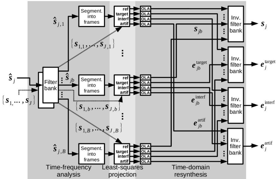
Figure 3: Block diagram of the proposed algorithm for the decomposition of an estimated source into the sum of the target source and three distortion components corresponding to target distortion, interference and artifacts.
