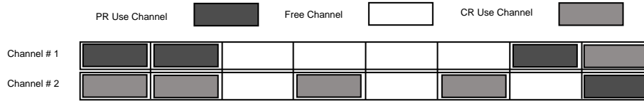
Figure 2: PR and CR Nodes occupancy over channels
