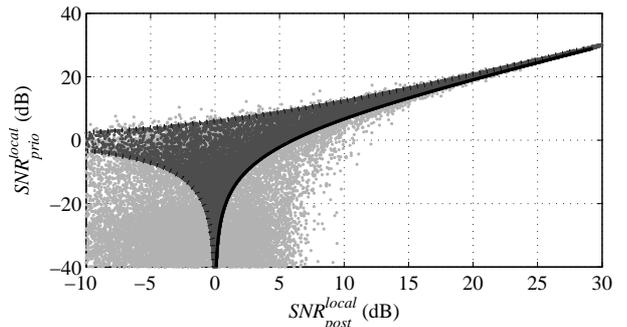
Figure 1:  $SNR_{prio}^{local}$  versus  $SNR_{post}^{local}$ . Dark gray features: clean speech and noise amplitudes are known in (6) and (7). Light gray features: clean speech amplitude is known but estimated noise PSD is used in (6) and (7).
