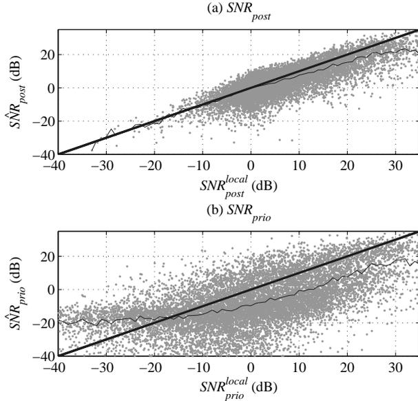
Figure 2: Estimated SNR versus true SNR (*i.e.* local SNR) in case of (a) *a posteriori* SNR and (b) *a priori* SNR. The bold line represents a perfect estimator and the thin line represents the mean of the estimated SNR versus the true SNR.
