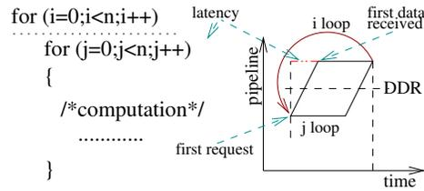
Figure 1: Latency penalty for an outer loop
