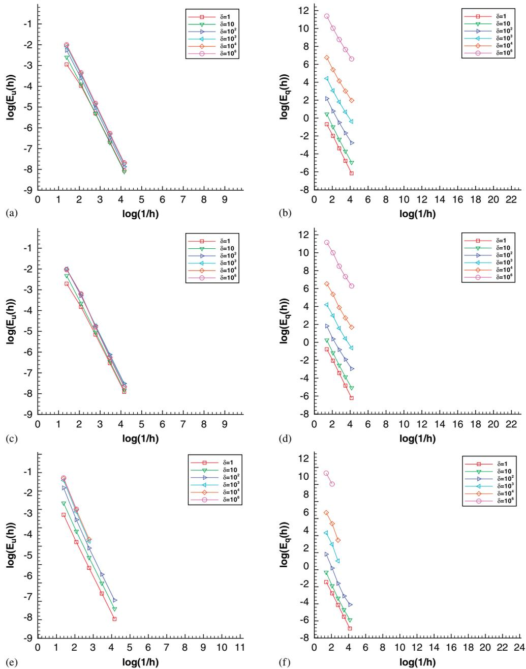
Figure 18. Test 5:  $L^2$  error curves for the scheme LPEW2 on the triangular mesh (Mesh1): (a) Case A: solution; (b) Case A: edge normal flux; (c) Case B: solution; (d) Case B: edge normal flux; (e) Case C: solution; and (f) Case C: edge normal flux.
