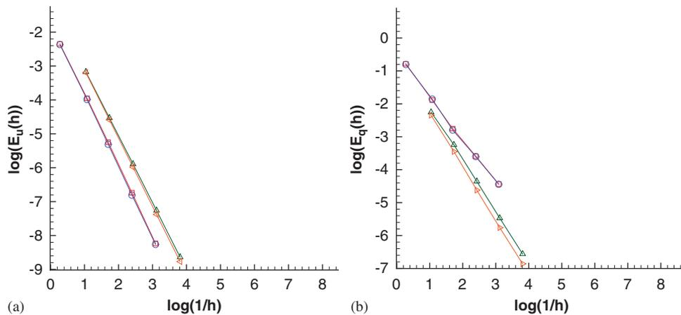
Figure 5. Test 1:  $L^2$  errors versus mesh size  $h$  for LPEW1 and LPEW2 on Mesh5 and Mesh6 with symbols:  $\Delta$  (LPEW1 on Mesh5),  $\triangleright$  (LPEW2 on Mesh5),  $\square$  (LPEW1 on Mesh6),  $\circ$  (LPEW2 on Mesh6): (a) solution and (b) edge normal flux.
