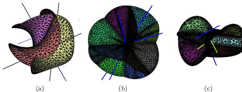
**Figure 2:** Diagrams are clipped by a sphere for convenience. (a) *VD* of 4 lines, obtained by rotating one line around the  $z$ -axis. All bisectors meet in that axis. (b) *VD* of 4 lines intersecting in one point. (c) *VD* of 4 lines, two lines intersect and the others are parallel to each of them, respectively.
