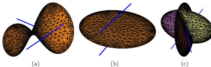
**Figure 1:** Bisector of: (a) two generic lines; (b) two parallel lines; (c) two intersecting lines. The diagrams were created with our implementation (see Section 5), and were clipped by a sphere for convenience.
