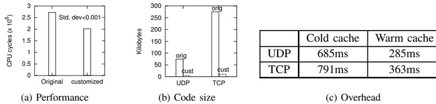
Fig. 4. Specialization results: Performance, code size and overhead.
