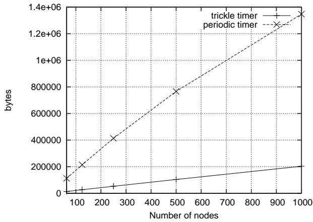
Figure 7: Total control traffic in bytes
