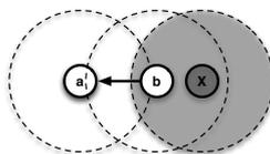
Figure 3: Unidirectional link due to radio interference
