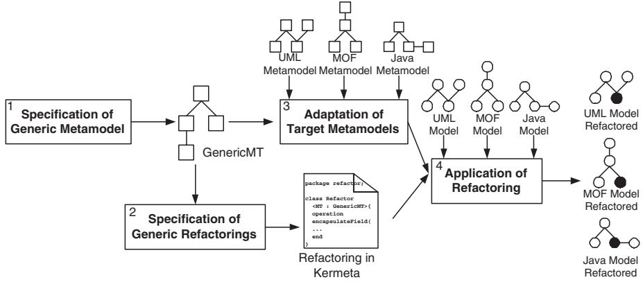
Fig. 7. Approach for the Specification of Generic Refactorings
