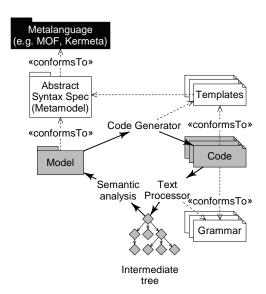
Figure 1: Typical concrete syntax definition and tooling
