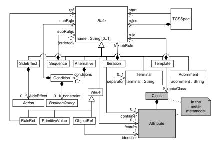
Figure 8: Overview of the meta-model for concrete syntax
