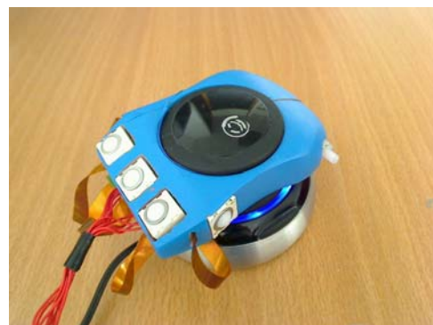
(b) The V5 prototype integrates only trackballs.
