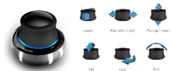
Figure 3. The SpaceNavigator and its degrees of freedom.
