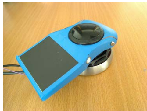
(a) The V4 prototype integrates a touchpad for the fingers except the thumb and a trackball on each side for the thumb.
