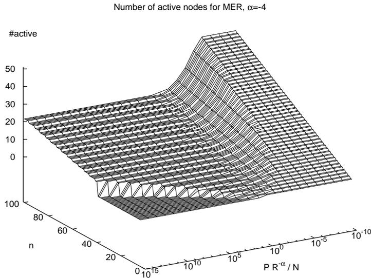
Figure 10: Number of nodes transmitting at the same time (inverse of  $s$ ) for MER. For large  $n$  it converges to between 4 and 5 nodes. Since distance between active nodes grows with power, DIR will have the same scheduling behavior for large powers. Note that the flow length does not change scheduling policy for minimal energy routing, but only total rate.
