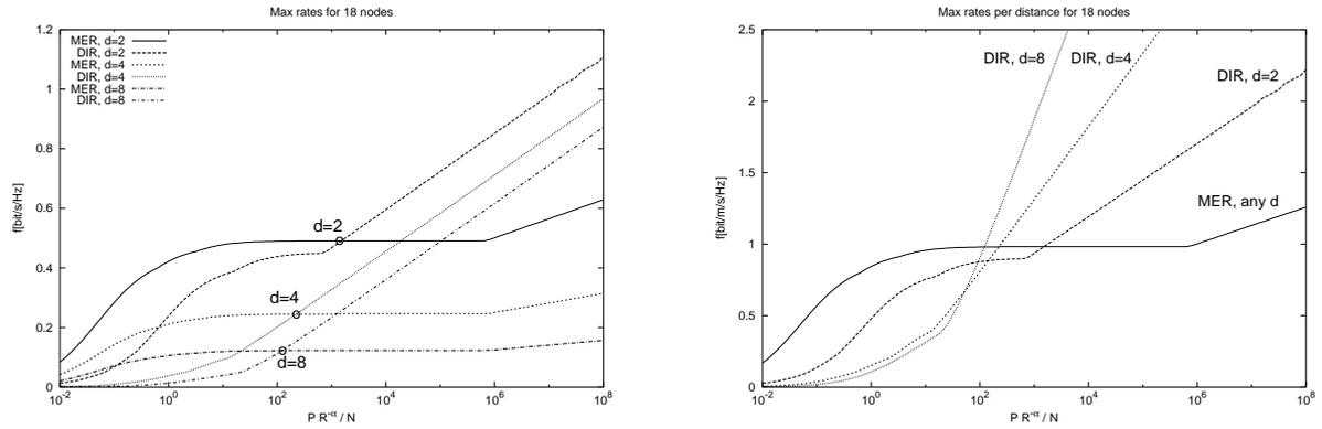
Figure 4: On the left, maximum rates for DIR and MER routing and different values of  $d$  are depicted, for a ring of 18 nodes. We see that for small transmitting powers MER routing is better than DIR, and for large powers DIR becomes better. The transition power depends on  $d$ . On the right, maximum rate per distance is depicted. We see that rate per distance is the same for MER, regardless of  $d$ . This is not the case for DIR.
