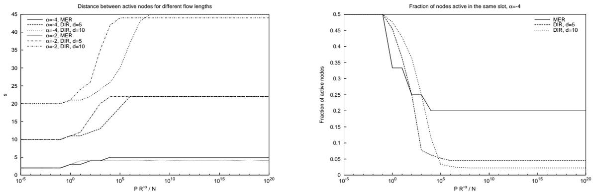
Figure 11: On the left is the average distance  $s$  between adjacent groups of active nodes. For small powers,  $s$  is 2 for MER and  $2d$  for DIR. It converges to approximately 4.5 for MER and  $4.5d$  for DIR. On the right is the fraction of nodes that are active in the same slot, which is directly proportional to dissipated energy.
