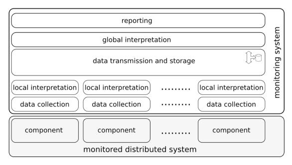
Figure 7.2: Architectural elements of a monitoring system
