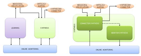
(a) Monitoring as a supporting functionality for learning and syn- (b) Feedback loop between CONNECTor synthesis and monitorthesis
