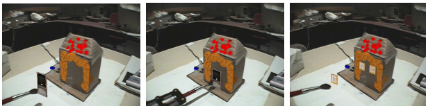
Figure 9: Interactive placement of labels: Left and middle – placement of a virtual door on a real house; right - placement of a window with the “label and copy” tool.
