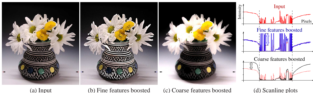
Figure 1: Our multiscale decomposition of image (a) allows detail to be extracted based on spatial scale rather than contrast and preserves edges. (b) Boosting fine scale features increases the contrast of the pattern on the vase. (c) Boosting coarse scale contrast and suppressing fine features reduces the contrast of the pattern, while increasing the contrast of the vase with its background. (d) Scanline plots (rows indicated using arrows in (a), (b) and (c)), illustrating the effect of the two equalizations (b) and (c). The dashed lines in the plots show two examples of edges that have been preserved.
