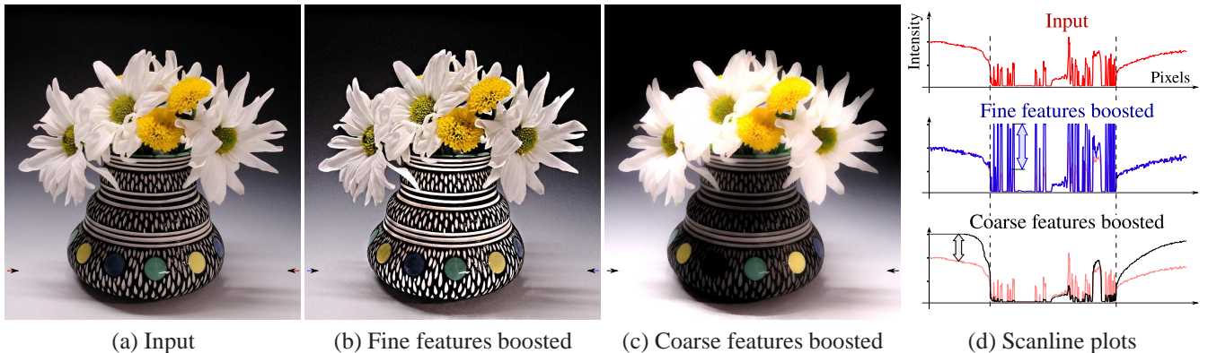
Figure 1: Our multiscale decomposition of image (a) allows detail to be extracted based on spatial scale rather than contrast and preserves edges. (b) Boosting fine scale features increases the contrast of the pattern on the vase. (c) Boosting coarse scale contrast and suppressing fine features reduces the contrast of the pattern, while increasing the contrast of the vase with its background. (d) Scanline plots (rows indicated using arrows in (a), (b) and (c)), illustrating the effect of the two equalizations (b) and (c). The dashed lines in the plots show two examples of edges that have been preserved.
