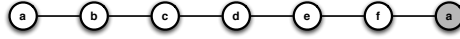
Figure 16: Identity Spoofing: the gray malicious router spoofs the identity of router a .
