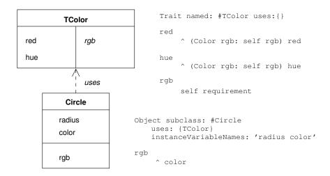
**Figure 1.** The trait TColor provides some methods shown in left column and requires the method in right column. The Circle class is enhanced with TColor behaviors by using the trait and providing a state and the required method. Equivalent Smalltalk code is given
