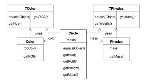
**Figure 6.** Using simultaneously TPhysics and TColor traits is a case for conflict, as both provides equals method with their own meaning. For Circle class, the problem can be solved by containing each implementation in a delegate class and providing a meaningful interface, either delegating, merging, excluding behaviors from delegates
