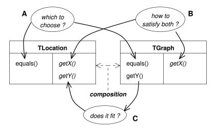
**Figure 9.** Three cases for conflicts in trait composition. When combining together TGraph and TLocation, the programmer should dismiss conflicts and meaningless links by carefully examining the situation. (A) Which behavior to choose for equals? One of both or a merge of both or nothing? (B) Does TLocation and TGraph share the same requirement when asking for getX? (C) Is the getY implementation from TGraph convenient for the requirement of TLocation?
