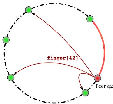
Figure 1: Example Chord DHT Ring.
