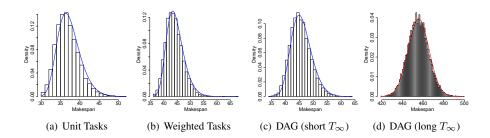
Figure 2: Distribution of the makespan for unit independent tasks 2(a), weighted independent tasks 2(b) and tasks with dependencies 2(c) and 2(d). The first three models follow a gev distribution (blue curves), the last one is gaussian (red curve).
