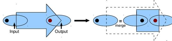
Figure 6: Example of connection transformer describing how a UP connection (**input**) whose **user** role is filled with a `CcmReceptacle<DataPush>` port can be seen as a UP connection (**output**) whose **provider** role is filled with a `CcmFacet<DataPull>` port. It does so by inserting a component instance acting as a cache.
