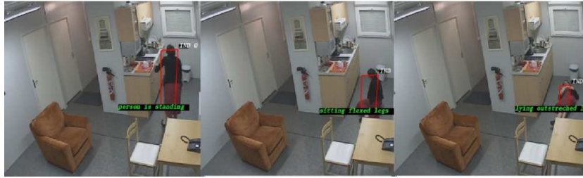
Fig. 8. Recognition of the "falling down" event
