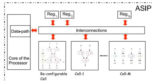
Figure 1. Generalized ASIP processor model.
