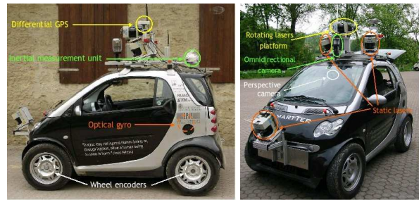
Fig. 5. The SmartTer passenger car equipped for autonomous driving. Behind the windscreen we have the camera system, on the sides of the roof we have the tilted laser scanners for corner protection. Currently, the front Sick has been replaced by an Alasca Scanner
