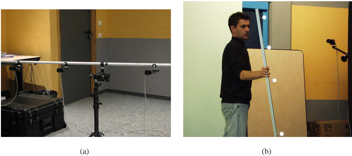
Figure 2: (a): Partial view of a 30-camera setup. (b): The calibration data are gathered by moving a one-dimensional object in the common field of view of the cameras.
