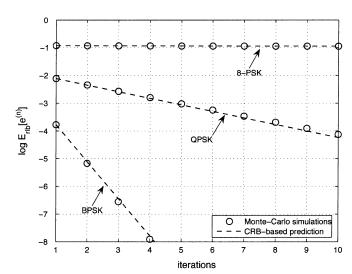
Fig. 4. Absolute mean distance between the ML estimate and the EM-algorithm estimate at a given iteration. Monte Carlo simulations are compared with the performance predicted by (58). The plot illustrates the sensitivity of the EM-algorithm speed of convergence to the choice of the constellation size.
