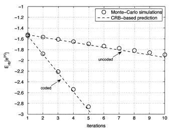
Fig. 8. Mean distance between the ML estimate and the EM-algorithm estimate at a given iteration. Monte Carlo simulations are compared with the performance predicted by (58). The plot illustrates the EM-algorithm speed of convergence for QPSK uncoded and coded transmissions.
