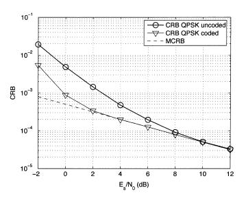
Fig. 6. CRBs versus  $E_s/N_0$ -ratio for QPSK uncoded and coded transmissions.
