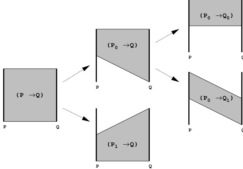
Figure 7: Building a hierarchy on the line space from an object  $P$  to an object  $Q$ . Starting with all lines from  $P$  to  $Q$  ( $P \rightarrow Q$ ) first the sender  $P$  is subdivided, resulting in new nodes  $(P_0, Q)$  and  $(P_1, Q)$ . These nodes in turn can be subdivided by splitting the receiver  $Q$  and so forth.
