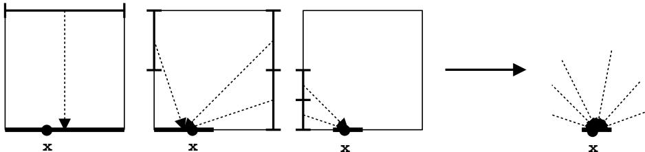
Figure 5: Links arriving at a some point  $x$  for a 2D box scene. For each link an illumination sample is added to the patches. These samples are then used as illumination description at the patch (right).
