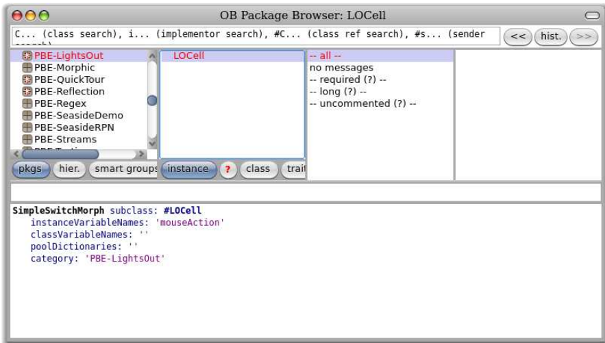
Figure 2.5: The newly-created class LCell
