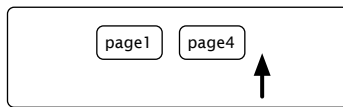
Figure 10.11: From page 1, the user clicks on a link to page 4. The history forgets pages 2 and 3.
