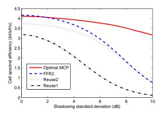
Fig. 4. Cell spectral effiency for 1D system, in function of the shadowing standard deviation, experiencing a path loss exponent.  $\alpha = 3$ .
