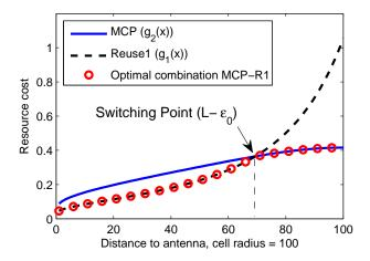
Fig. 2. Resource needs vs distance to BS. Black dashed line: standard transmission with 1 antenna  $g_1(x)$ ; blue solid line: 2x1 MCP transmission  $g_2(x)$  and red circles: optimal combination of both.
