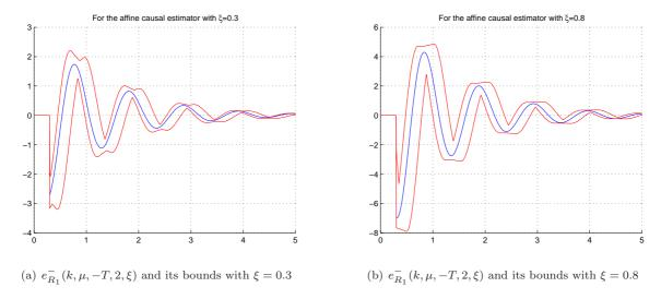
Figure 2: Comparisons between the bias term errors for the affine causal estimator and their bounds
