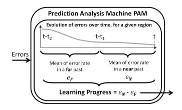
Fig. 1. Internal mechanism of the Prediction Analysis Machine PAM associated to a given subregion R of the sensorimotor space. This module considers errors detected in prediction by the Prediction Machine PM, and returns a value representative of the learning progress in the region. Learning progress is the derivative of errors analyzed between a far and a near past in a fixed length sliding window.
