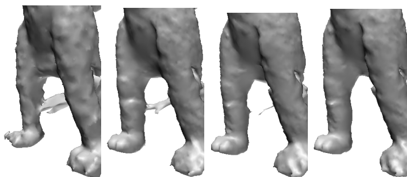
Figure 15: Example of topological changes during in 3-D reconstruction for the dinosaur sequence, introduced in Figure 14. The start-up surface, obtained from triangulated 3-D points via PowerCrust [6] contains several topological errors (i.e. the extra branch connecting the dinosaur's limbs). They are corrected during the surface evolution, as shown in the right most image.
