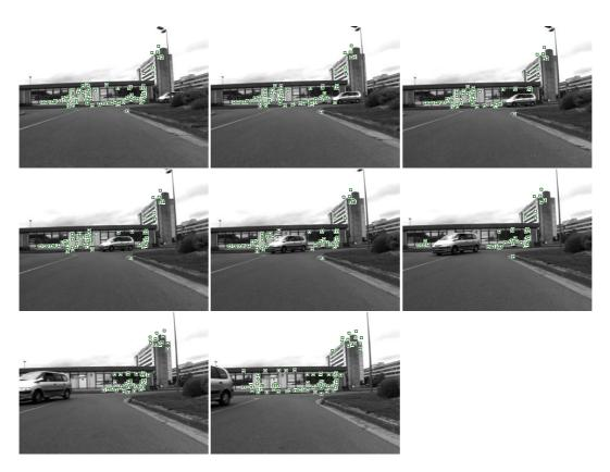
Fig. 19. Sequence of images obtained during the execution of a navigation experiment. The points used for navigation re-appear after being occluded and dis-occluded by a moving car. This is possible since the localization component is able to predict the locations of the invisible features and consequently re-start their tracking on the fly.
