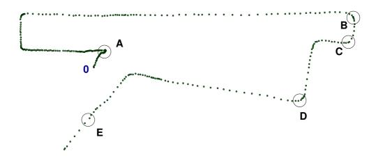
Fig. 18. The graph of 320 nodes mapping a  $1.1 \,\mathrm{km}$  reference path which was considered in one of the control experiments. Large circles mark places where initializations took place. Between the points A and B the robot drove approximately 740 m without human intervention.
