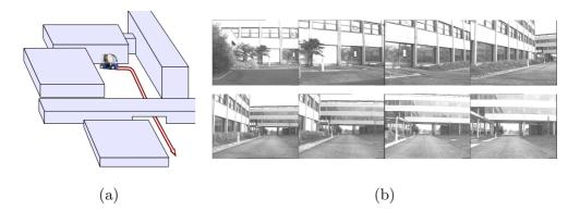
Fig. 1. Appearance-based navigation with a perspective camera: the sketch of a navigation task (a), and the set of first eight images from the environment representation forming a linear graph (b). Note that the graph has been constructed automatically using the mapping component described in 5.1.2.
