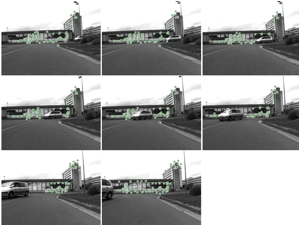
Fig. 19. Sequence of images obtained during the execution of a navigation experiment. The points used for navigation re-appear after being occluded and dis-occluded by a moving car. This is possible since the localization component is able to predict the locations of the invisible features and consequently re-start their tracking on the fly.
