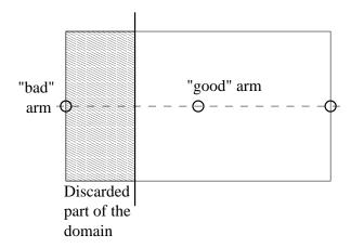
**Fig. 2.** The large rectangle is the domain  $[x_n^-, x_n^+]$ . The three circles are arms  $x_n' x_n' x_n' x_n' x_n'$ ; the left arm is the "bad" arm, whereas the arm in the center is the "good" arm, *i.e.* the one which proved to be closer to the optimum than the left arm, with confidence  $1 - 6\delta/(\pi^2 n^2)$ .
