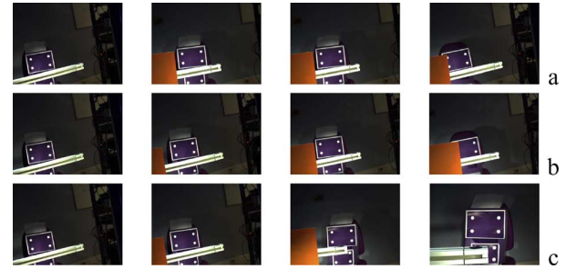
Fig. 17. Experiment C: main phases of the servo (a) without avoidance, (b) with the avoidance law projected using the classical redundancy formalism, and (c) using the directional redundancy. The pictures are taken by the embedded camera. The visual target is the four-white-points rectangle. The occluding object is the orange shape that appears in the left of the image.
