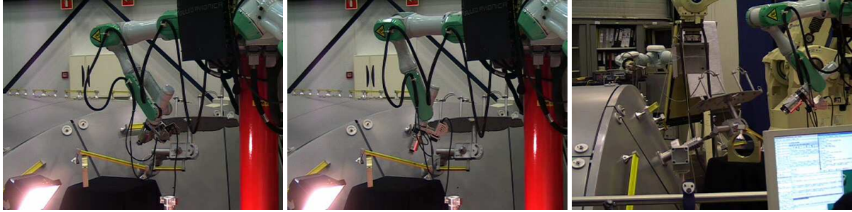
Figure 12: External view of a visual servoing experiment on an handrail at ESA/ESTEC using the Eurobot prototype. The APFR used in the other experiment is also attached to the mockup behind the robot. First image shows the robot at its initial position. In the second image the robot is parallel to the handrail. In the last image the robot is in grasping position.
