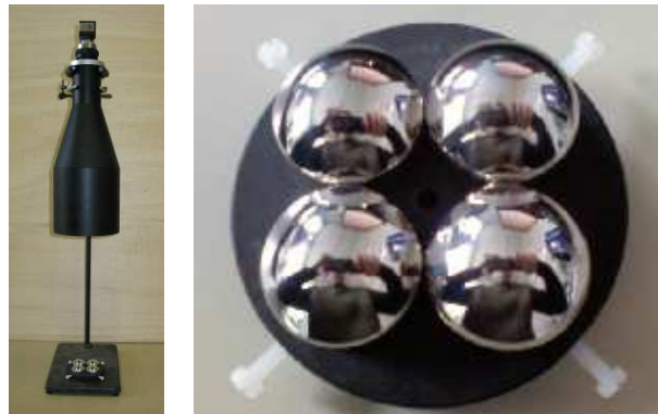
Fig. 1. Our sensor: orthographic camera, parabolic mirrors, 90 cm height
