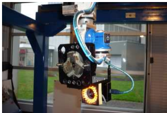
Fig. 7. Camera and light-ring mounted on the robot end-effector.
