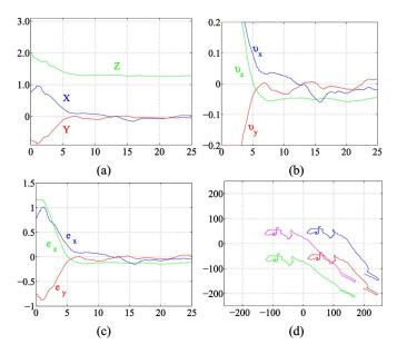
Fig. 4. Results obtained for  $\boldsymbol{v}=0.4\mathrm{e}$ : time evolution (in seconds) of the real position in the task space (in meters), (a) of them velocity output of the visual servo control  $\boldsymbol{v}$  (in meters per seconds) (b). The evolution of the visual error is plotted on (c), and the trajectory of the four black marks in the image plane are plotted in (d).
