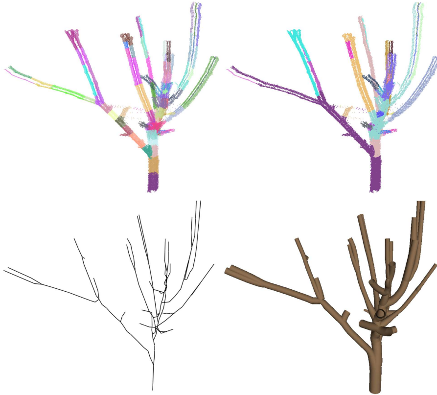
Figure 6: Reconstruction result of fagus. Top: Segmentation and branch detection result. Bottom: Skeleton and the lofting result.
