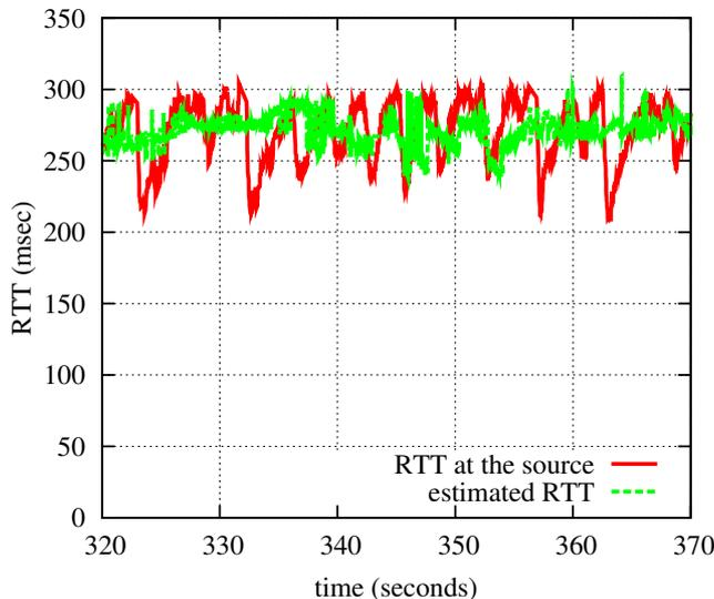
Figure 6: Example of the RTT measured at the source and the estimated RTT (exp2).
