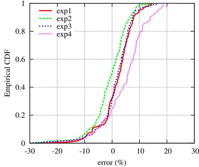
Figure 8: Empirical CDF of the error between the RTT measured at the source and the estimated RTT (testbed).
