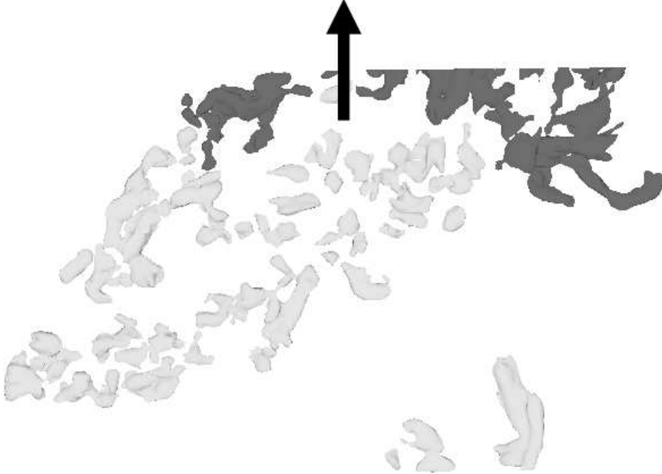
Fig. 4. Distribution of extracted components. Finished components are shown in light grey and growing ones in dark grey. The black arrow indicates the direction used for extraction.
