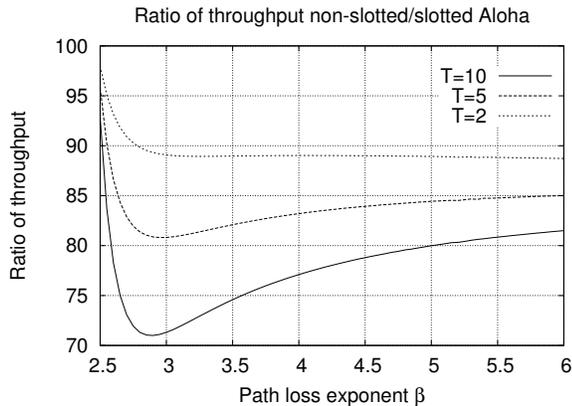
Fig. 1. The ratio (in %) of the good-put offered by the non-slotted Aloha with respect to the slotted one, as a function of the path loss exponent  $\beta$ , for various choices of the SINR threshold  $T$ ; other parameters are  $p = \frac{\epsilon}{1+\epsilon} = 0.05$ ,  $\lambda = 0.001$ ,  $r = \sqrt{1000}$ .
