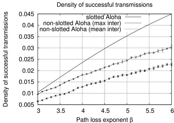
Fig. 5. Density of successful transmissions versus path loss exponent  $\beta$ . Slotted Aloha and non-slotted Aloha (mean and maximal interference constraint) are tuned to maximize the density of successful transmissions.
